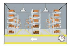
After elapse of hold time, the sensor switches off the light when no motion is detected.
