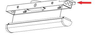
3. Fix the lamp body on the wall by screws, complete the installation; repeat the previous procedure to install the 3rd strip light, 4th strip light etc.
