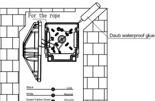
2) Fix the cover of driver and waterproof cotton pad on the wall.
