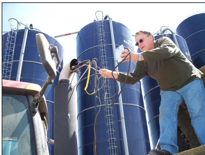
The above photograph shows one method in which exhaust pressure can be monitored during the Carbon Balance test procedure. In this case, exhaust pressure is ascertained through the use of a Magnahelic gauge. This type of stringent regime further documents the inherent accuracy of the Carbon Balance test.
