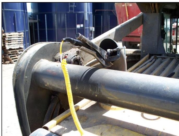
Once the exhaust temperature has stabilized, the test unit has reached its peak operating temperature. Exhaust temperature is critical to the completion of a successful evaluation, since temperature changes identify changes in load and RPM. As previously discussed, RPM and load must remain constant during the Carbon Balance study.
