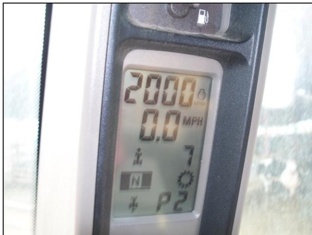
Once engine fluid levels have reached normal operating conditions the Carbon Balance study may begin. The above photograph shows that the engine RPM is locked in place at 2000 r.p.m. It should be noted that any deviation in r.p.m., temperature, either fluid or exhaust, would cause this unit to be eliminated from the evaluation due to mechanical inconsistencies.
