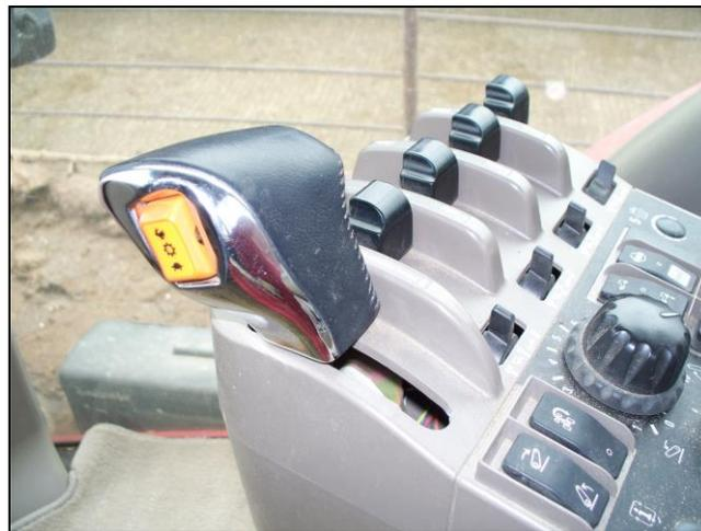
A factory throttle position lock is utilized, as one method, to secure engine RPM. This provides a steady state condition in which consistent data can be collected. Should the engine RPM fluctuate erratically and uncontrollably, the test unit would be disqualified from further consideration.
