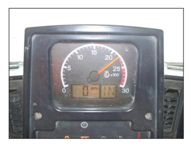
Once engine fluid levels have reached optimal operating conditions the Carbon Mass Balance study may begin. Although, for the purpose of this procedure, all test units were evaluated at full throttle, the above photograph identifies the target engine speed, on one of the test units, at full throttle (2200 RPM). It should be noted that any deviation in RPM, temperature, either fluid or exhaust, would cause this unit to be eliminated from the evaluation due to mechanical inconsistencies.
