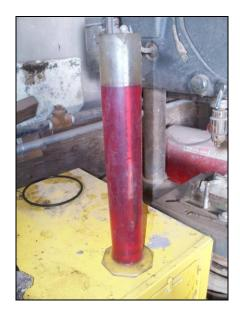
Fuel density and temperature tests are performed for both the baseline and treated segments of the evaluation to determine the energy content of the fuel. A .800 to .910 Precision Hydrometer, columnar flask and Raytek Minitemp are used to determine the fuel density for each prescribed segment of the evaluation.
