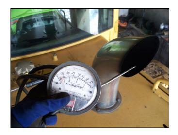
The above photograph shows one method in which exhaust pressure can be monitored during the Carbon Mass Balance test procedure. In this case, exhaust pressure is ascertained through the use of a Magnahelic gauge. This type of stringent regime further documents the inherent accuracy of the Carbon Mass Balance test.
