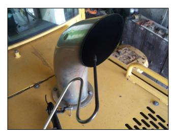
While the emission-sampling probe is in place, and data is being collected, exhaust temperature and pressure are monitored throughout the entirety of the Carbon Mass Balance procedure. This photograph shows the typical location of the exhaust emissions sampling probe.
