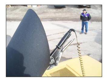
Once the exhaust temperature has stabilized the test unit has reached its peak operating temperature. Exhaust temperature is critical to the completion of a successful evaluation since fluctuating temperatures identify changes in load and RPM. As previously discussed, RPM and load must remain constant during the Carbon Mass Balance study.
