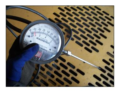
The same data was collected for air inlet velocities. This procedure is utilized to ensure that engine air inlet velocities are not restricted during the course of the evaluation. This process helps to prevent an artificially lean to rich or converse performance condition.
