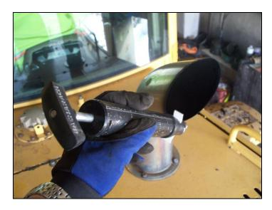
The above photograph demonstrates a typical method in which soot particulate volume is monitored during the Carbon Mass Balance test. This method is the Bacharach Smoke Spot Test. It is extremely accurate, portable, and repeatable. It is a valuable tool in smoke spot testing when comparing baseline (untreated) exhaust to the Fuel Factor X catalyst treated exhaust.
