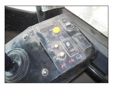
A factory equipped throttle control or an individual depressing the throttle pedal to the full throttle position are implemented as a means to secure engine RPM. This provides a steady state condition in which consistent data can be collected. Should the engine RPM fluctuate erratically and uncontrollably, the test unit would be disqualified from further consideration.
