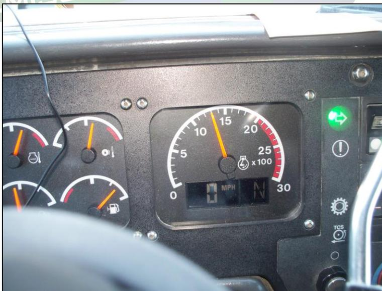
Once engine fluid levels have reached normal operating conditions the Carbon Mass Balance study may begin. The above photograph shows that the engine RPM is locked in place at 1300 RPM. It should be noted that any deviation in RPM, temperature, either fluid or exhaust, would cause this unit to be eliminated from the evaluation due to mechanical inconsistencies.
