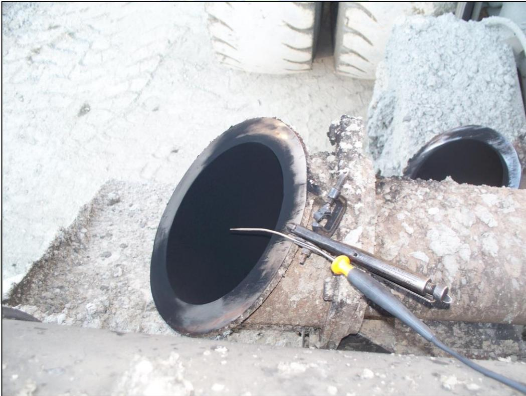
Once the exhaust temperature has stabilized, the test unit has reached its peak operating temperature. Exhaust temperature is critical to the completion of a successful evaluation, since temperature changes identify changes in load and RPM. As previously discussed, RPM and load must remain constant during the Carbon Mass Balance study.
