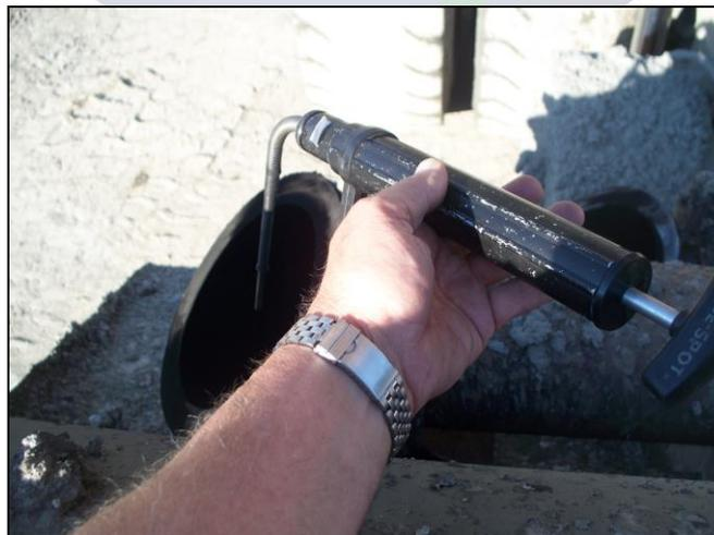
The above photograph demonstrates a typical method in which soot particulate volume is monitored during the Carbon Mass Balance test. This method is the Bacharach Smoke Spot test. It is extremely accurate, portable, and repeatable. It is a valuable tool in smoke spot testing when comparing baseline (untreated) exhaust to catalyst treated exhaust.
