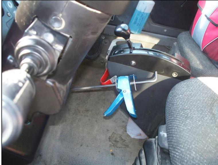
An aftermarket throttle position lock is utilized, as one method, to secure engine RPM. This provides a steady state condition in which consistent data can be collected.
