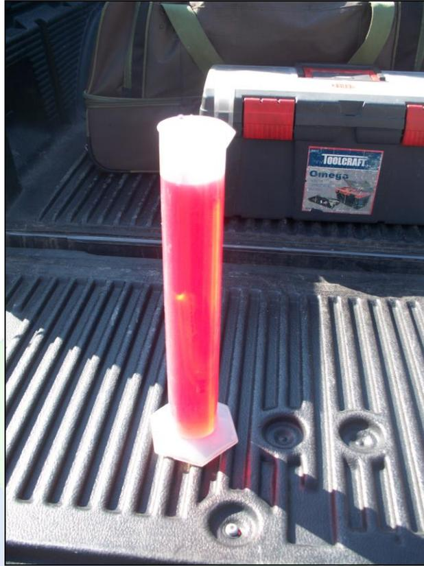
Fuel density and temperature tests are performed for both the baseline and treated segments of the evaluation to determine the energy content of the fuel. A .800 to .910 Precision Hydrometer, columnar flask and Raytek Minitemp are utilized to determine the fuel density for each prescribed segment of the evaluation.
