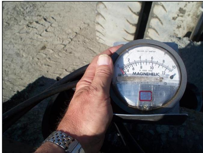
The photograph above and below identifies one method in which exhaust pressure and air inlet velocity can be monitored during the Carbon Mass Balance test procedure. In this case, exhaust pressure and air inlet velocity are ascertained through the use of a Magnahelic gauge. This type of stringent regime further documents the inherent accuracy of the Carbon Mass Balance test.
