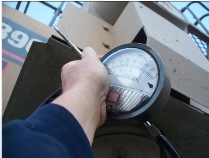
At the conclusion of the Carbon Mass Balance test, a soot particulate test is performed to determine the engine exhaust particulate level. This valuable procedure helps to determine the soot particulate content in the exhaust stream. Soot particulates are the most obvious and compelling sign of high emissions levels. Any attempt to reduce soot particulates places all industry in a favorable position with environmental policy as well as the general public.
