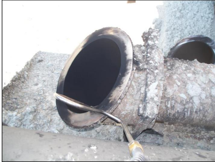
While the emission-sampling probe is in place, and data is being collected, exhaust temperature and pressure are monitored throughout the entirety of the Carbon Mass Balance procedure. This photograph shows the typical location of the exhaust emissions sampling probe.
