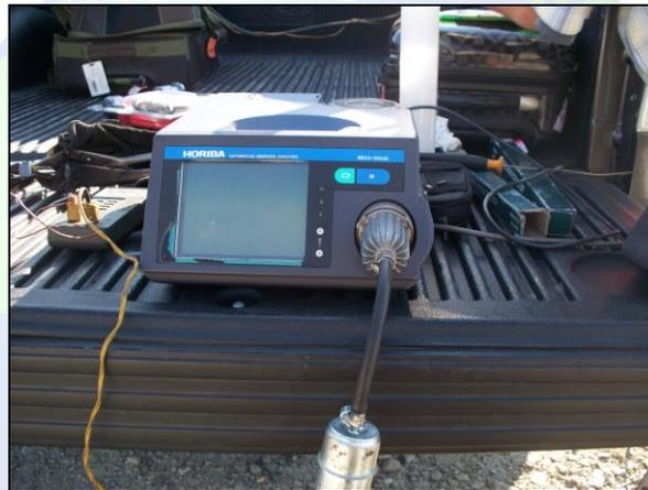
The above photograph identifies one type of analyzer used to perform the Carbon Mass Balance test. The analyzer is calibrated with known reference gases before the baseline and treated test segments begin.
