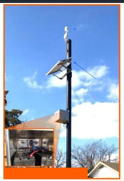
• ALL other nodes are powered by solar (minimum 24V)
