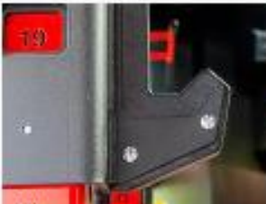
Elevated UHMW Channel eliminates metal-on-metal contact.
