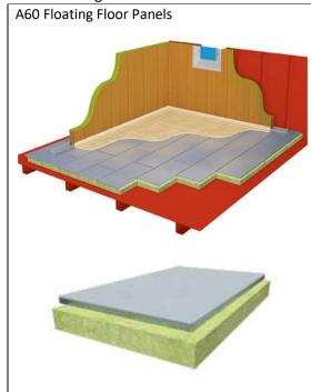
Panel: **ENSAR Floating Floor Panels** Type: 2mm thick Galvanised Steel
