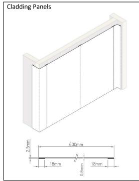
Panel: **PVC Coated Mild Steel** Folded Long Edges Type: Overall Thickness: 0.6mm (Sheet)
