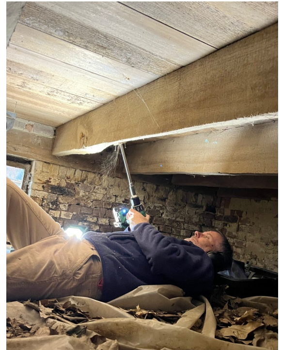
Dendrochronologist Michael Worthington taking sample from Gate House floor beams
