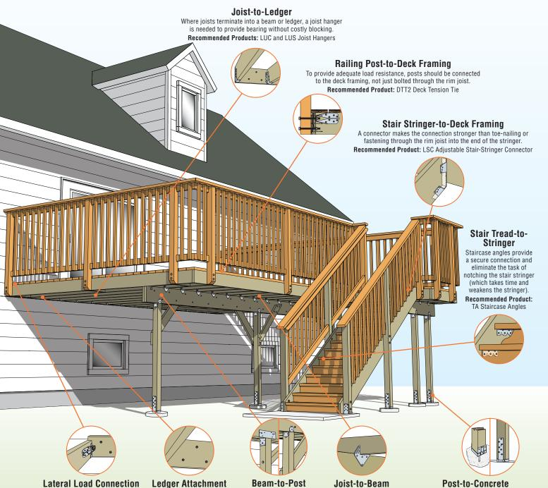
In some applications it is necessary to reinforce the connection to the adjacent house to resist lateral (side-to-side) movement. A connection back into the floor joists is the recommended method.
