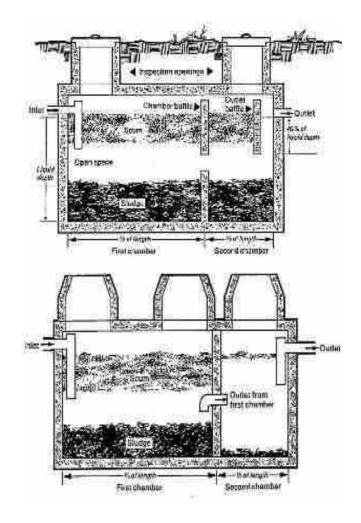
This USDA sketch of a different two-compartment septic tank design illustrates how additional compartments can help retain solid waste in the septic tank and improve the quality of wastewater discharged to the drainfield or soakaway bed or absorption bed.
