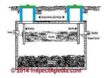
You may also notice that our septic tank shown above has inlet and outlet baffles constructed of concrete while the septic tank below shows an inlet baffle constructed using plastic pipe - a common repair method if septic tank baffles are damaged.
