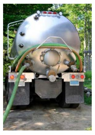
Wipes can also clog the vacuum hose that service providers use to pump the tank. Removing clogs, whether they are in the tank or the vacuum hose, makes routine servicing of septic tanks take longer. Longer service times means greater costs for the pumper—costs that naturally get passed on to the homeowner.
