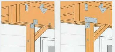
At the point where a beam meets a post, it must be properly connected to the post in order to resist gravity, lateral and uplift loads. This pertains to solid sawn beams or those comprised of multiple members, whether they rest on top or are fastened to the side of the post.
