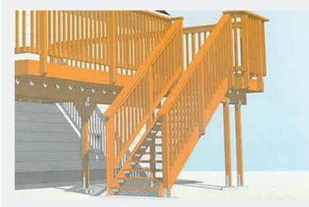
Stair stringers must be connected to the deck, and treads properly connected to the stringers, in order to resist loads. In addition, code requirements regarding openings between stairs treads and stair railings must also be met.
