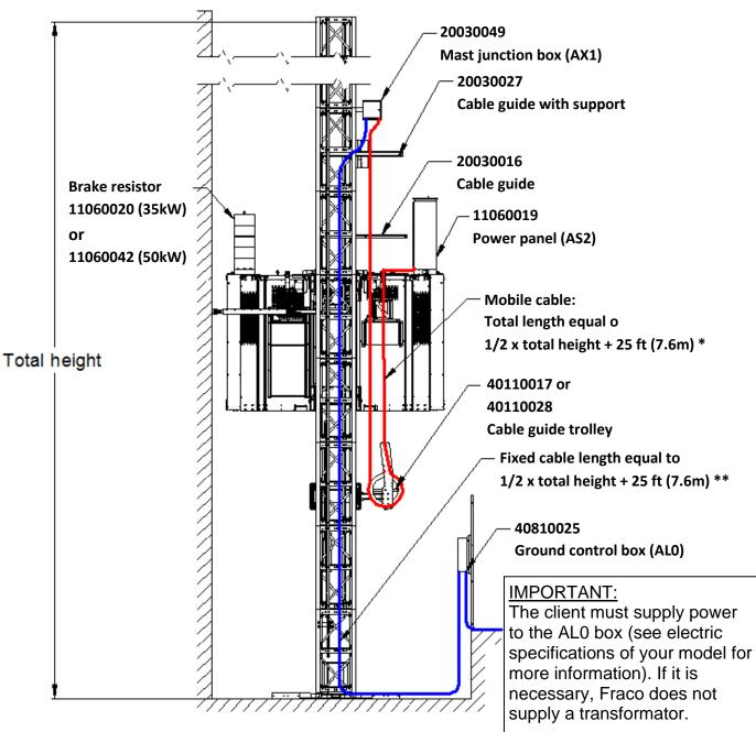
\* Mobile cable must be type *DRAKA INDUSTRITE, 4 strands* (Strands dimension depend on model). Any other type of cable must be approved by Fraco to be used. \*\* No special requirement for cable type.
