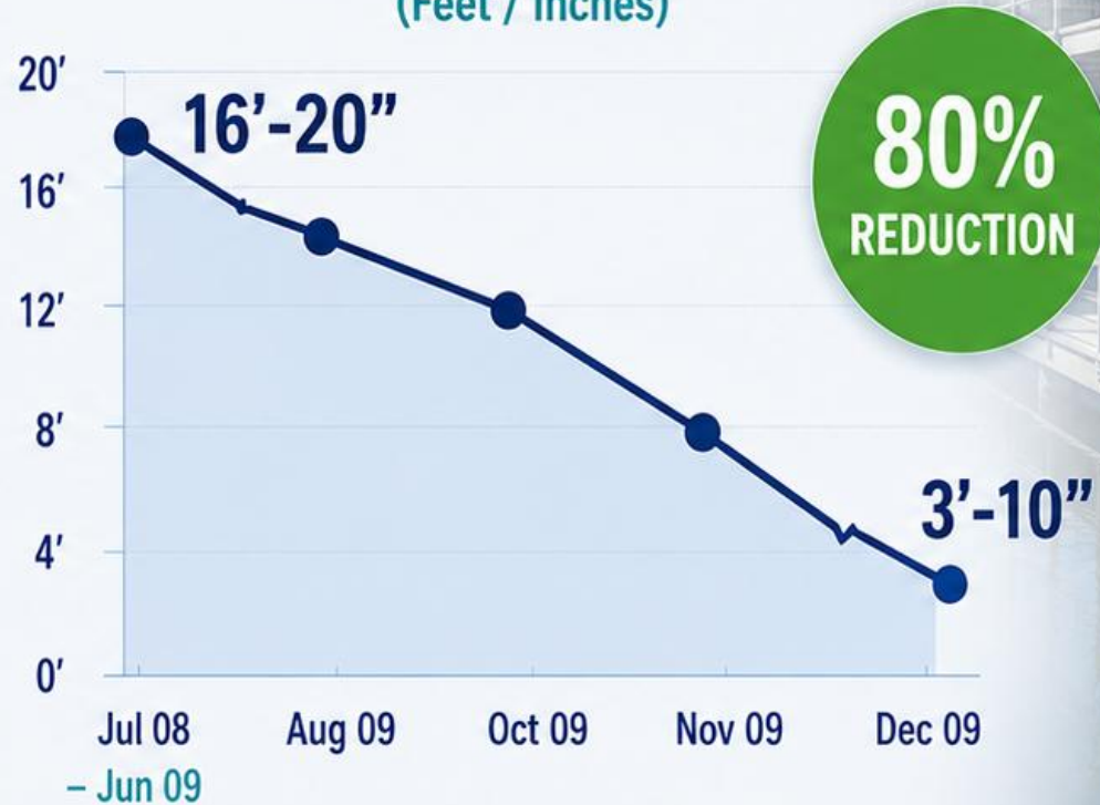
Reduction in sludge level in storage tanks (Feet / Inches)
