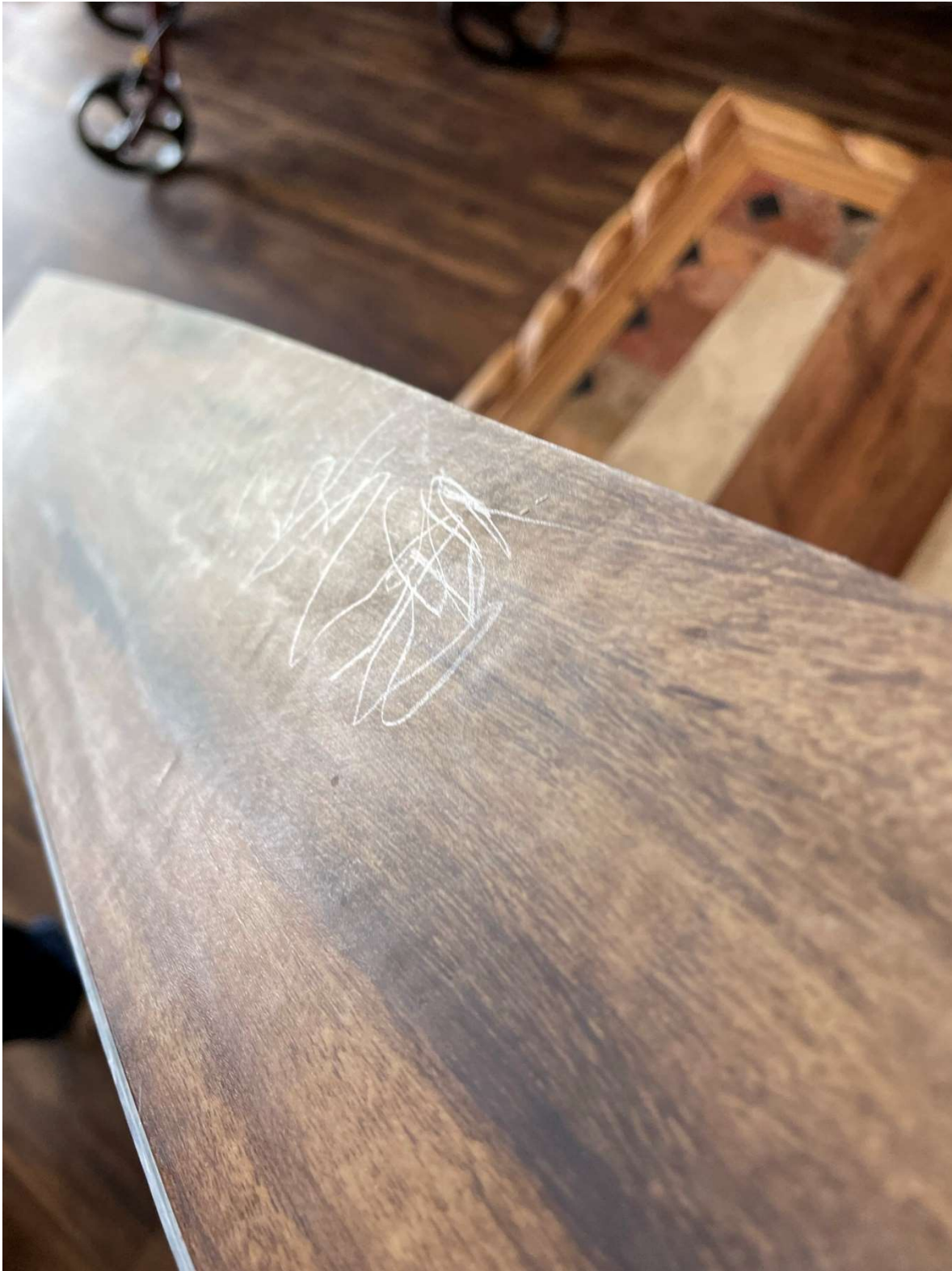
Scuff marks in wear layer- Made with customer's fingernail for demonstration.
