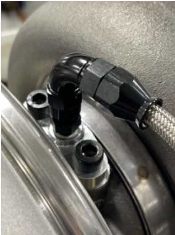
-4AN PTFE 90 degree to the turbo feed fitting
