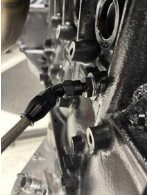
-4AN PTFE 45 degree to engine block oil feed.
