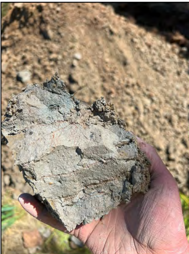
Image 5 (left) and Image 6 (right): Image 5 depicts typical blocky excavated texture and indurated character of the native undifferentiated glacial deposits as observed in the majority of our explorations. Image 6 depicts conditions in TP-11, with topsoil over weathered glacial deposits (undifferentiated) over glacial deposits (undifferentiated). Note seepage collecting in base of excavation.
