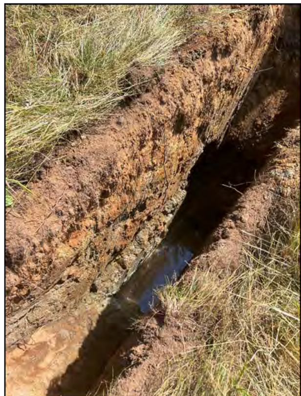
Image 5 (left) and Image 6 (right): Image 5 depicts typical blocky excavated texture and indurated character of the native undifferentiated glacial deposits as observed in the majority of our explorations. Image 6 depicts conditions in TP-11, with topsoil over weathered glacial deposits (undifferentiated) over glacial deposits (undifferentiated). Note seepage collecting in base of excavation.
