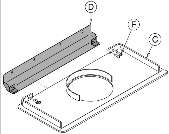
6. Install the step top and fix it in place using the screws **(B)** removed previously.
