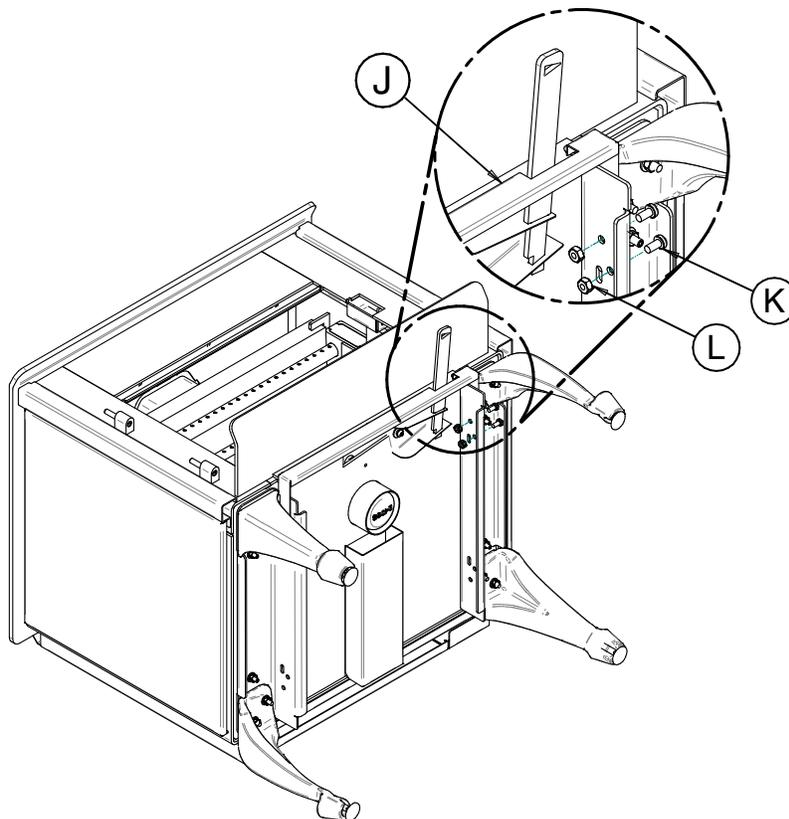
6. Put the stove on its legs, install the ash drawer included with the kit. Put back the firebricks, the ash plug and the door on the stove. See step 1.
