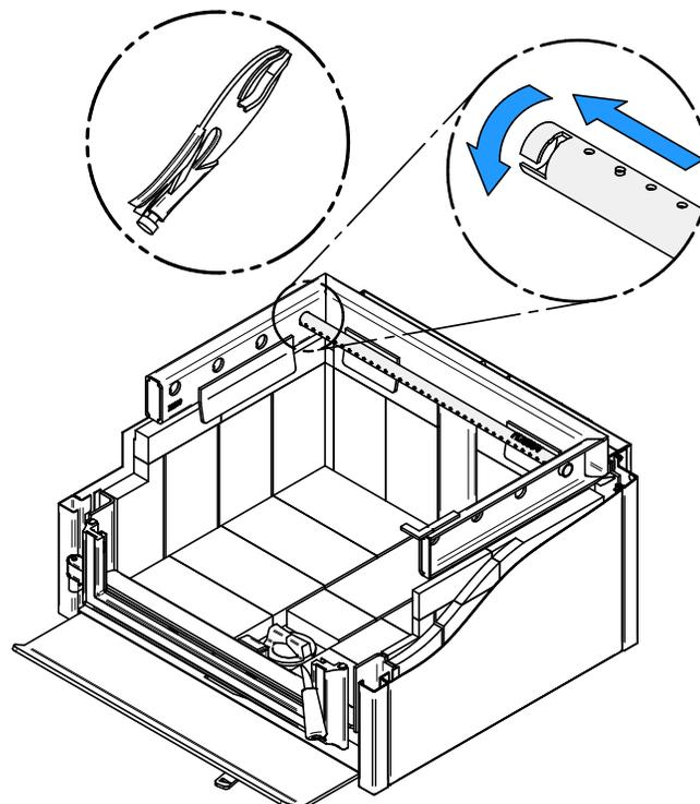
Note that secondary air tubes (A) can be replaced without removing the baffle board (B) and that all tubes are identical.
