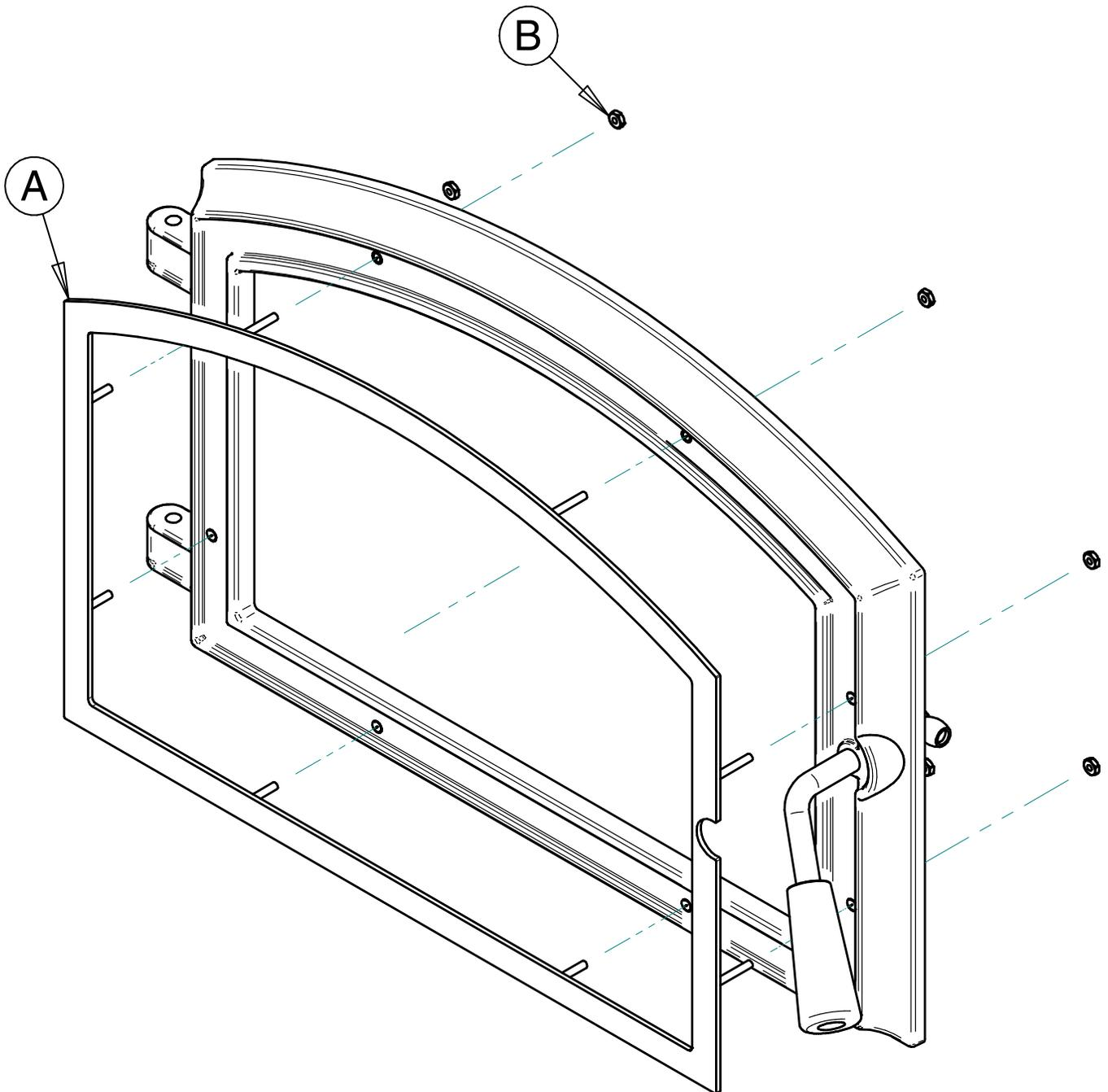
*Note: It is not necessary to remove the glass to install the overlay.*
