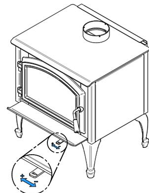
As the air intake is reduced, the flame slows down. If the flames diminish to the point of disappearing, the air intake has been reduced too early in the combustion cycle or the wood used is too wet. If the wood is dry and the air control is used properly, the flames should decrease, but remain bright and stable.
