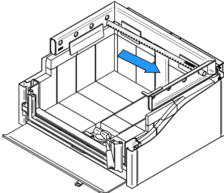
2. Align the notch in the left end of the tube with the key of the left air channel hole. Using a « Wise grip » hold the tube and lock it in place by turning the tube as shown. Make sure the notch reaches the end of the key way.
