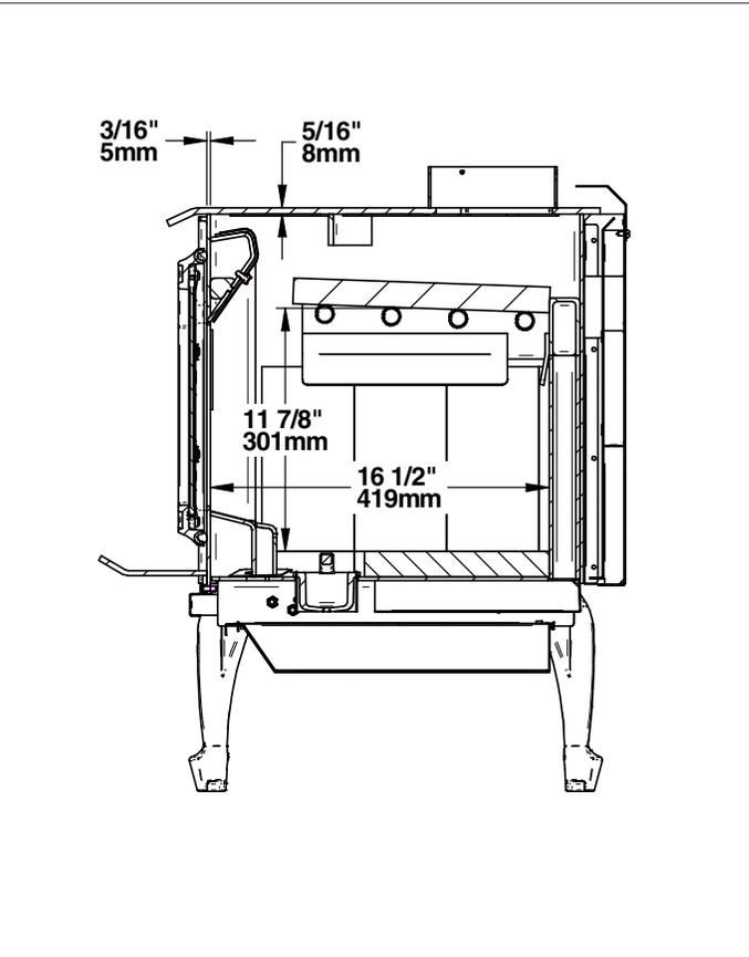
Figure 12: Side View - Combustion Chamber
