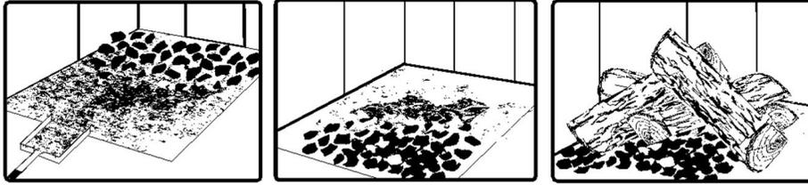
Close the air control only when the firebox is full of bright turbulent flames, the wood is charred, and its edges are glowing.
