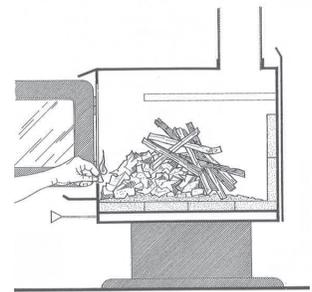
Once the fire has ignited, the door can be closed with the air control still fully open. When the kindling is almost completely burned, standard firewood pieces can be added.
