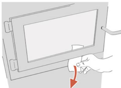
In order for the stove to burn at its best efficiency, the door must provide a perfect seal with the firebox. The tightness of the door seal can be verified by closing and latching the door on a strip of paper. The test must be performed all around the door. If the paper slips out easily anywhere, either adjust the door or replace the gasket.
