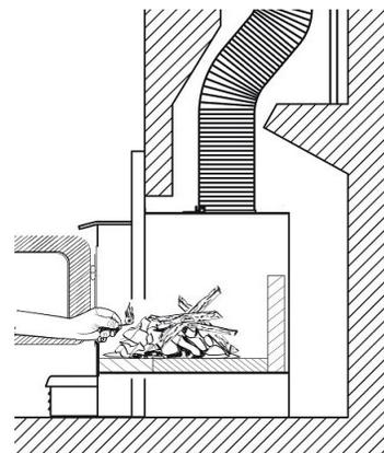
*Do not leave the insert unattended when the door is slightly open. Always close and latch the door after the fire ignites.*
