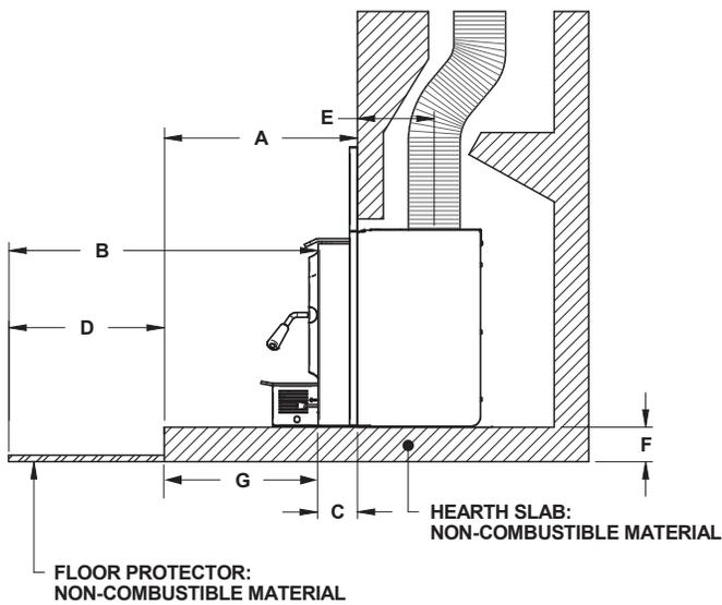
Figure 13: Additional Floor Protection - Raised Installation
