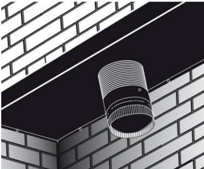
Figure 17: Block-off Plate
