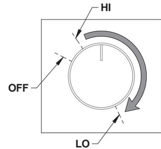
The insert is also equipped with a heat sensor who works with the blower. When the blower is on (position between LO and HI), the thermodisc will start the blower automatically when the insert is hot enough and it will stop it when the insert has cooled down. Therefore, the variable speed control can be left at the desired setting.
