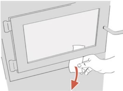
In order for the insert to burn at its best efficiency, the door must provide a perfect seal with the firebox. Therefore, the gasket should be inspected periodically to check for a good seal. The tightness of the door seal can be verified by closing and latching the door on a strip of paper. The test must be performed all around the door. If the paper slips out easily anywhere, either adjust the door or replace the gasket.
