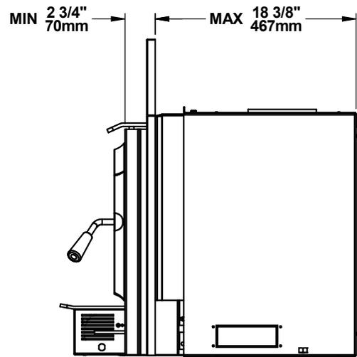
Figure 2: Side View - Minimum Insert Projection
