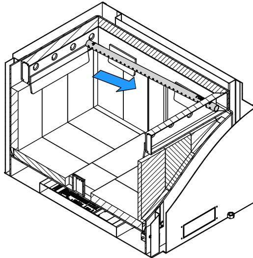
2. Align the notch in the left end of the tube with the key of the left air channel hole. Using a « Wise grip » hold the tube and lock it in place by turning the tube as shown. Make sure the notch reaches the end of the key way.
