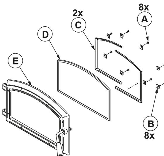
*The two main causes of broken door glass are uneven placement in the door and over-tightening the retaining screws.*
