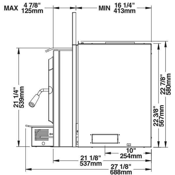
Figure 4: Side View - Maximum Insert Projection
