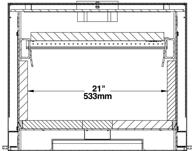
Figure 6: Front View - Combustion Chamber
