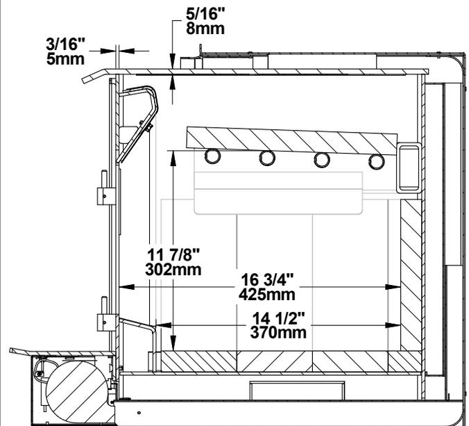
Figure 7: Side View - Combustion Chamber
