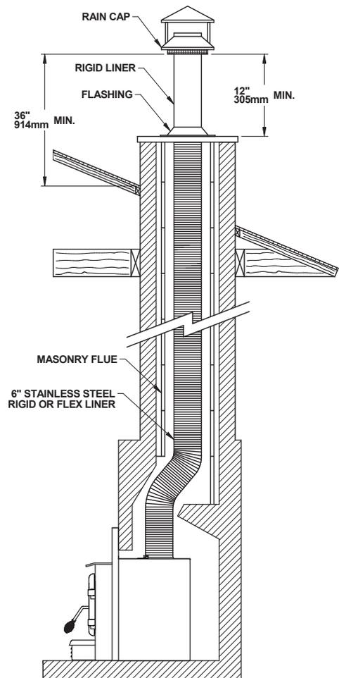
Figure 18: Liner Installation
