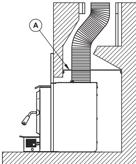
Figure 16: Block-off Plate
