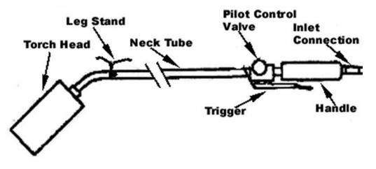
Figure 2: Basic components of a roofing torch
