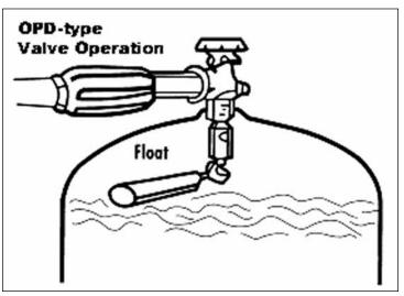
Figure 3: OPD valve operation
