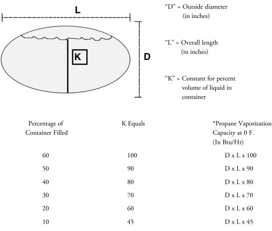
\*These formulas allow for the temperature of the liquid to refrigerate to -20 F, producing a temperature differential of 20 degrees for the transfer of heat from the air to the container's "wetted" surface and then into the liquid. The vapor space area of the vessel is not considered. Its effect is negligible.
