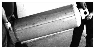
Photo 5: This is the proper way to carry a 100-pound cylinder.
