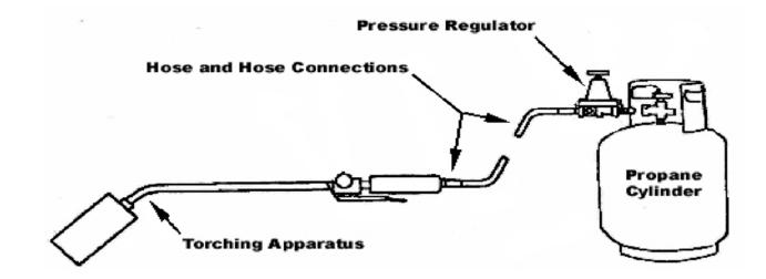
Figure 1: A complete roofing torch assembly
