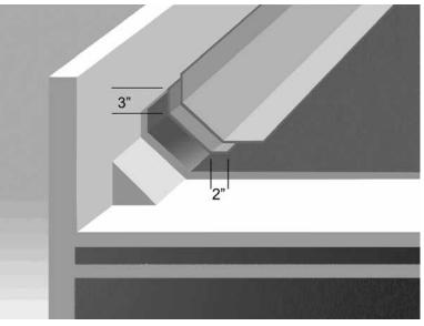
Figure 2: Extend backer layer 3 inches vertically and 2 inches horizontally.
