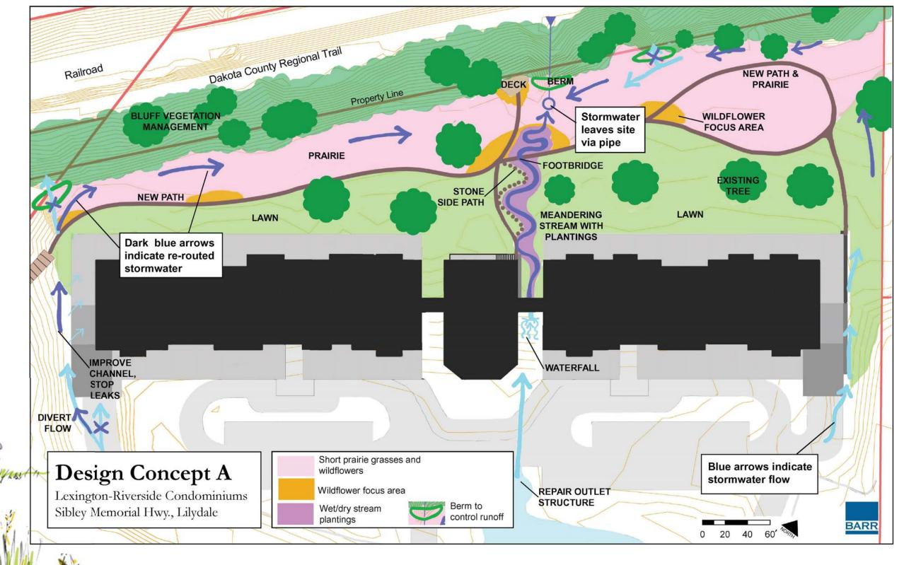
Stormwater retrofit concept, with sketch showing a meandering "stormwater stream." This feature, accepting runoff from a parking lot and other impervious areas, would infiltrate and slow water as well as create visual amenity at this environmentally sensitive site, perched on bluffs above the Mississippi.
