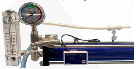
You may stack the membranes using the provided groove. 1/4" or 6mm
