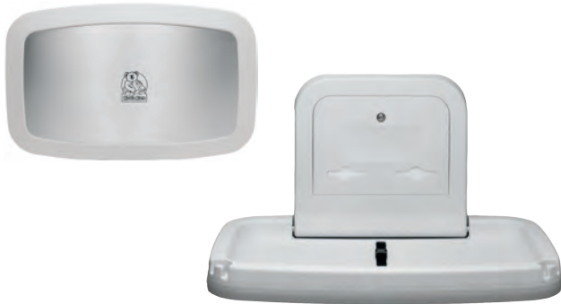
KB200-SS HORIZONTAL, WALL-MOUNTED WITH STAINLESS STEEL VENEER Polypropylene cabinet and bed with 22-gauge, Type-304 satin stainless steel veneer. Unit 35 3/16" W, 22 1/4" H. Depth (closed) 4". Extension (open) 23 3/16".
