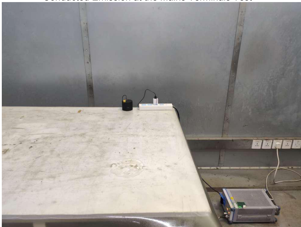
Conducted Emission at the Mains Terminals Test
