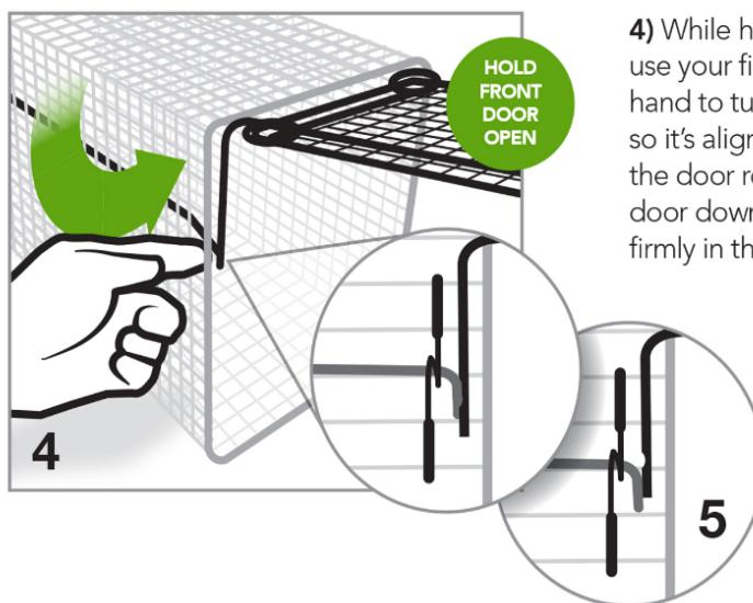
**4)** While holding the door open, use your finger with the opposite hand to turn the trigger rod up, so it's aligned with the groove of the door rod. Slowly move the door down, so the trigger rod rests firmly in the door rod groove.
