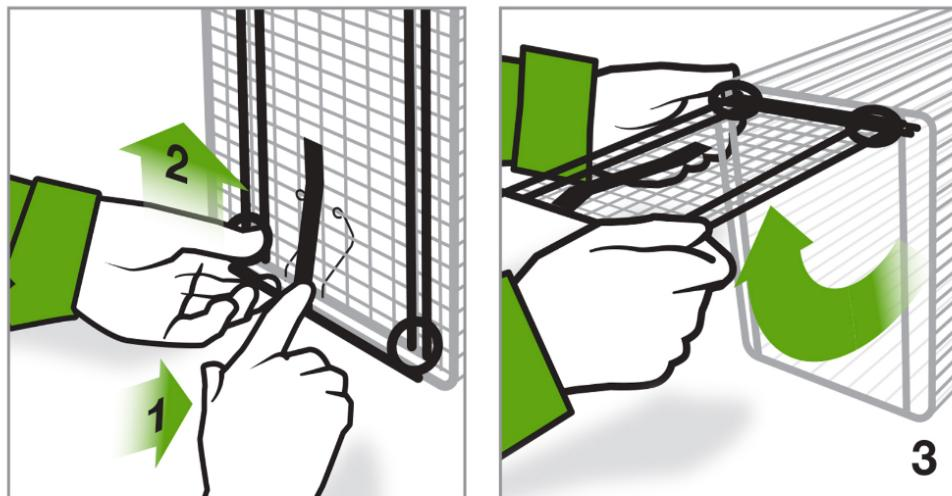
**1)** Push in front door lock and **2)** slide ring rod up to the top of the door.
