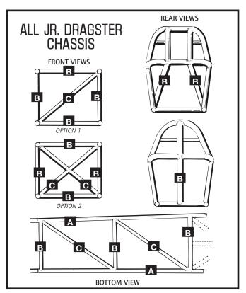
wire feed or TIG heliarc process. Welding must be free of slag and porosity. Any grinding of welds prohibited. Plating of chassis prohibited on all new vehicles.
