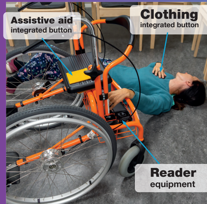
Fig. 2. Visualisation of a potential use scenario for passive RFID push buttons. Wearable nurse call and mobile reader equipment.
