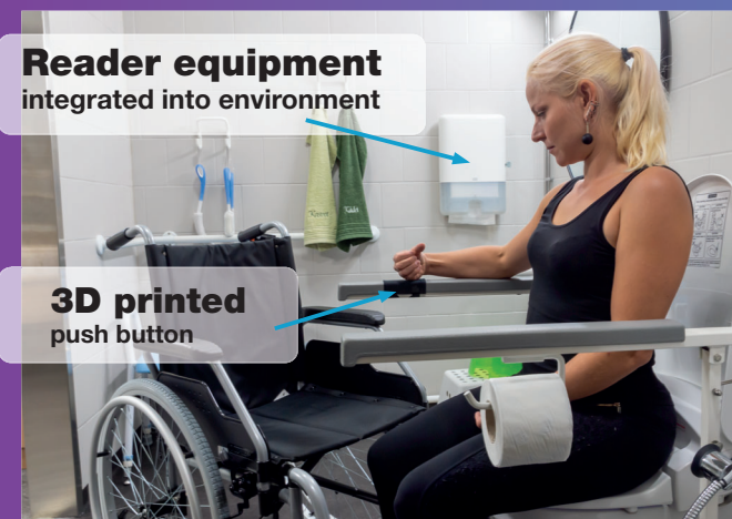
Fig. 3. Visualisation of a potential use scenario for passive RFID pushbuttons. Reader equipment integrated into the environment, in this case toilet in which the push-button is used to call for help.
