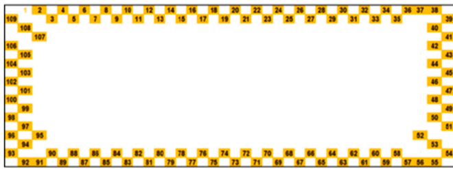
Fig. 12. Solder joint labelling scheme for the flip-chip packages.
