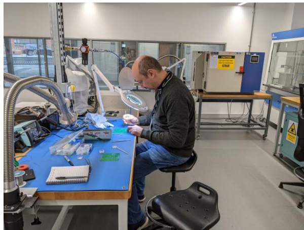
13 - SUT Pioneer placing solder balls on PCB
