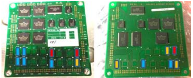
Fig. 10. 0.8-mm ENIG board layout with color-coded flip-chip positions based on reliability.
