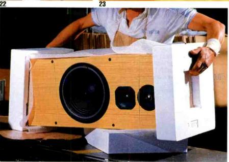
22-23. The cabinet's veneer is polished and the drizers are mounted in openings on the main parels during final assembly of the speaker.
