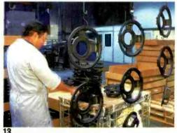
11-13. The cast frames for the L10013's woofers are electrostatically coated with an epoxy powder, which is then baked on, rather than being painted conventionally. One benefit is a pollution-free working environment.
