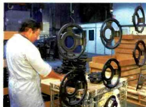
11-13. The cast frames for the L100t3's woofers are electrostatically coated with an epoxy powder, which is then baked on, rather than being painted conventionally. One benefit is a pollution-free working environment.
