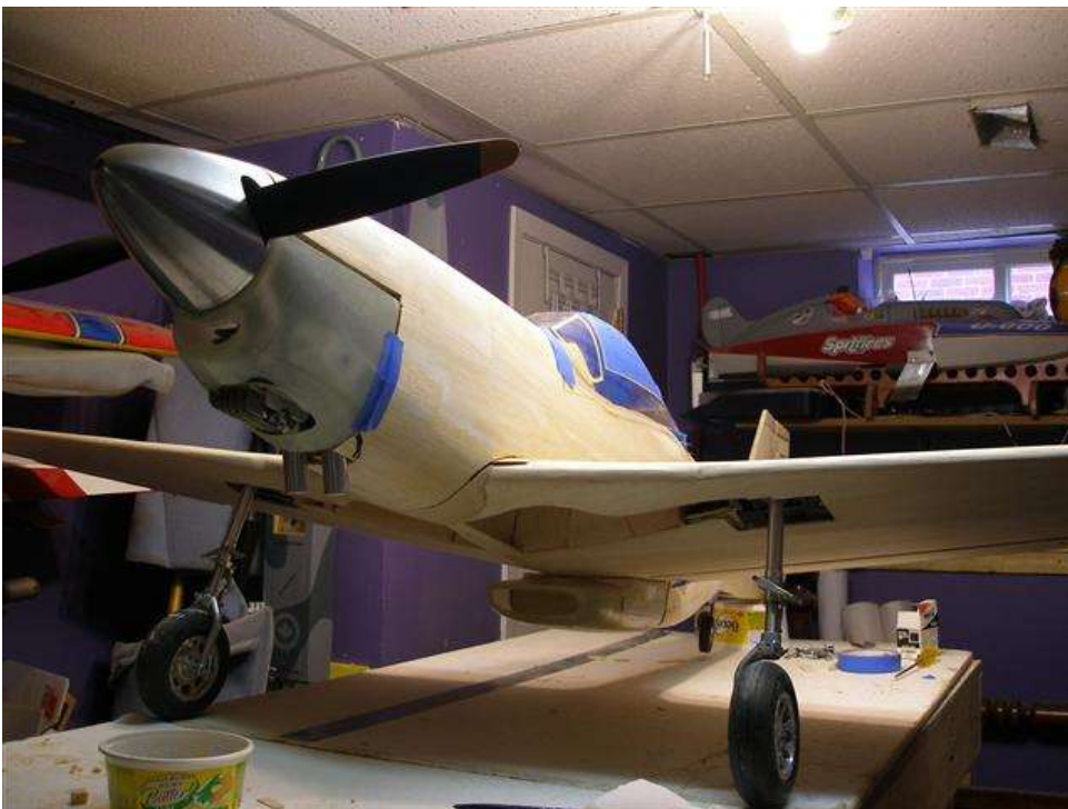
All together. This is the easy part. Next comes fiber glassing the entire fuselage and wing and finishing the detail parts.
