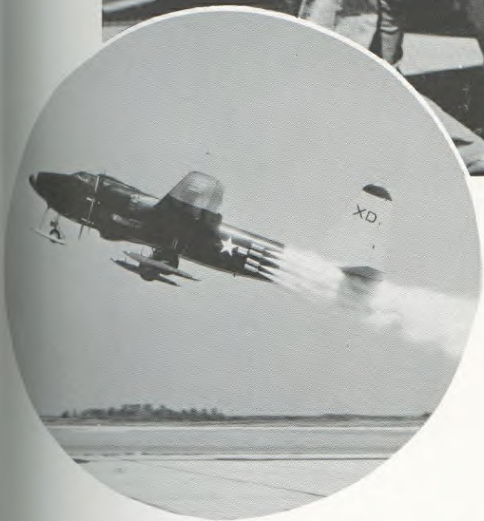
JATO, jet assist take-off, gets P2V off the ground in a hurry. Above, members of VX-6 being instructed in proper installation of Jato bottles carried on racks at side of plane. Only the larger planes carried this equipment.
