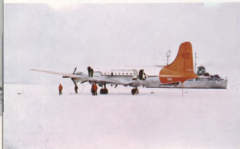
SKYMASTER, wheel-equipped R5D, a 4-motor workhorse for long-range reconnaissance and photo missions.
