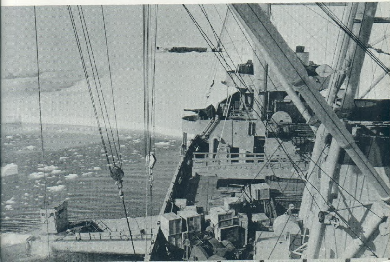
LCM "MIKE" BOAT SERVES AS TUG TO SHOVE SHIP ALONGSIDE BAY ICE AT LITTLE AMERICA V
