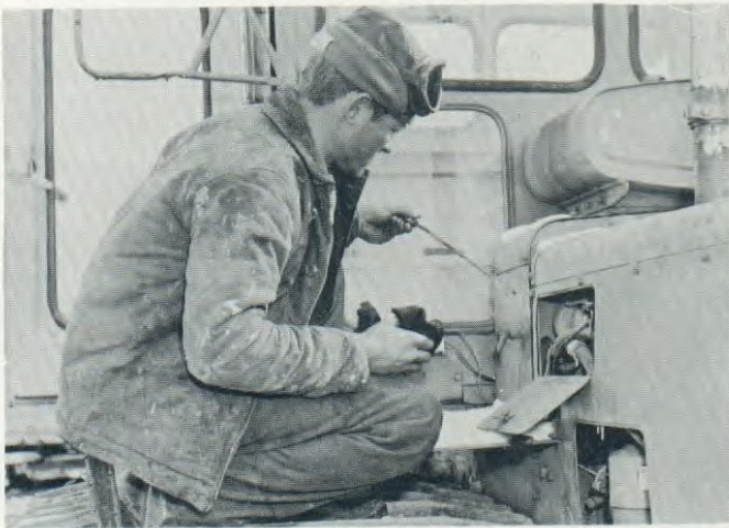
OIL CHECK is made on Caterpillar D-2 tractor by its chauffeur, Sidney G. Armistead, cm1, to keep it rolling.
