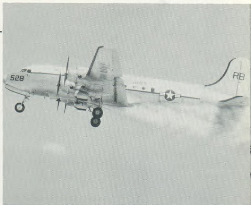
JET ASSIST take-off puts R5D Skymaster into the air within seconds of go signal for photo reconnaissance tour.
