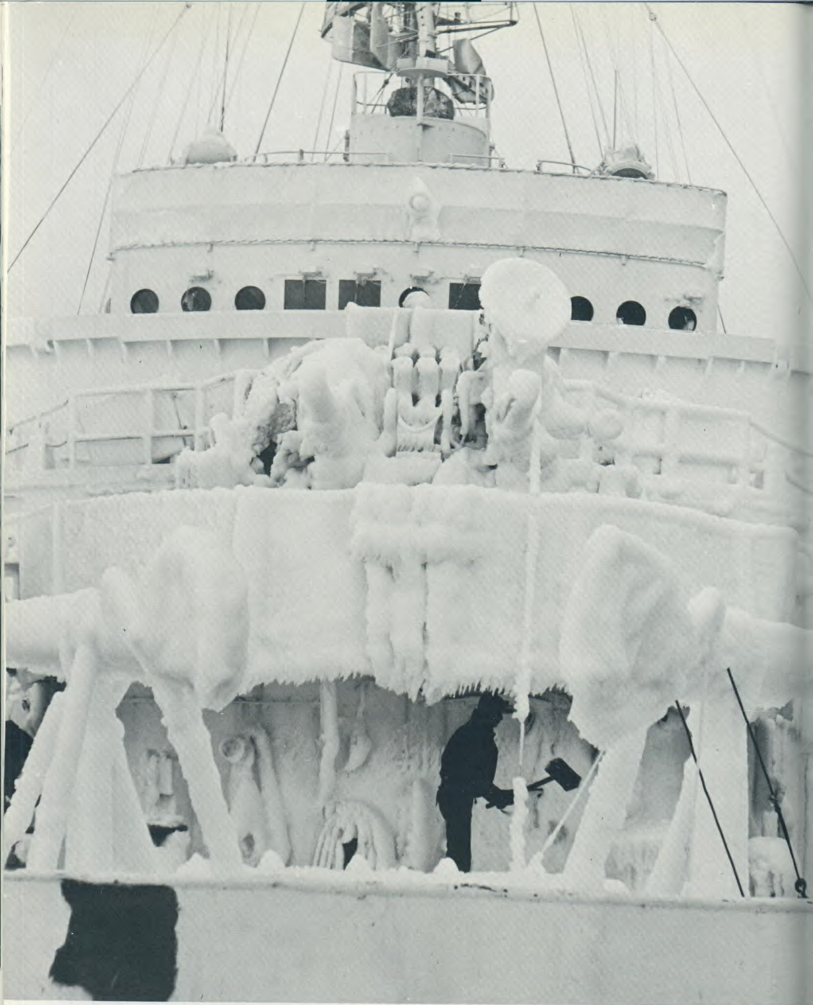
FROSTED LIKE A WEDDING CAKE, EASTWIND IS THAWED OUT BY CREWMEN USING STEAM, HAMMERS
