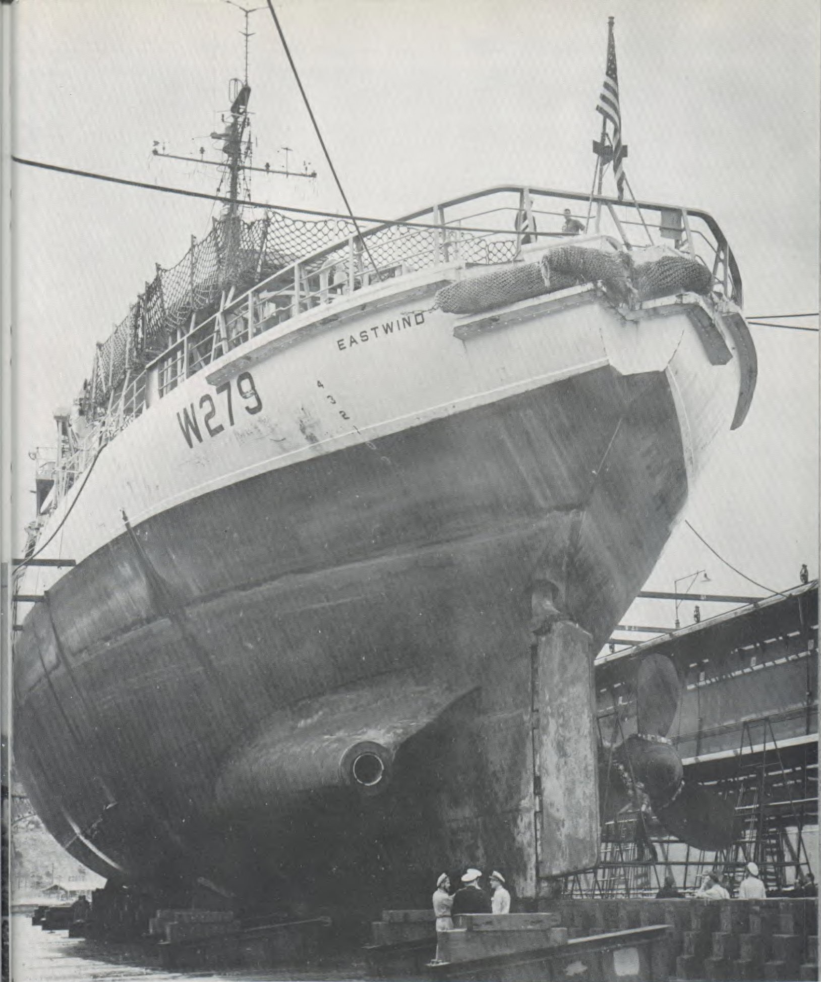
USS EASTWIND IN DRYDOCK AT WELLINGTON, N. Z. AS ONE REMAINING PROPELLER UNDERGOES REPAIR
