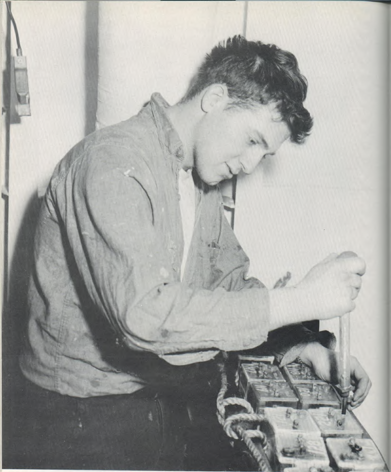
CREWMAN OF USS GLACIER TESTS BATTERY IN THE SHIP'S BATTERY LOCKER ABOARD ICEBREAKER
