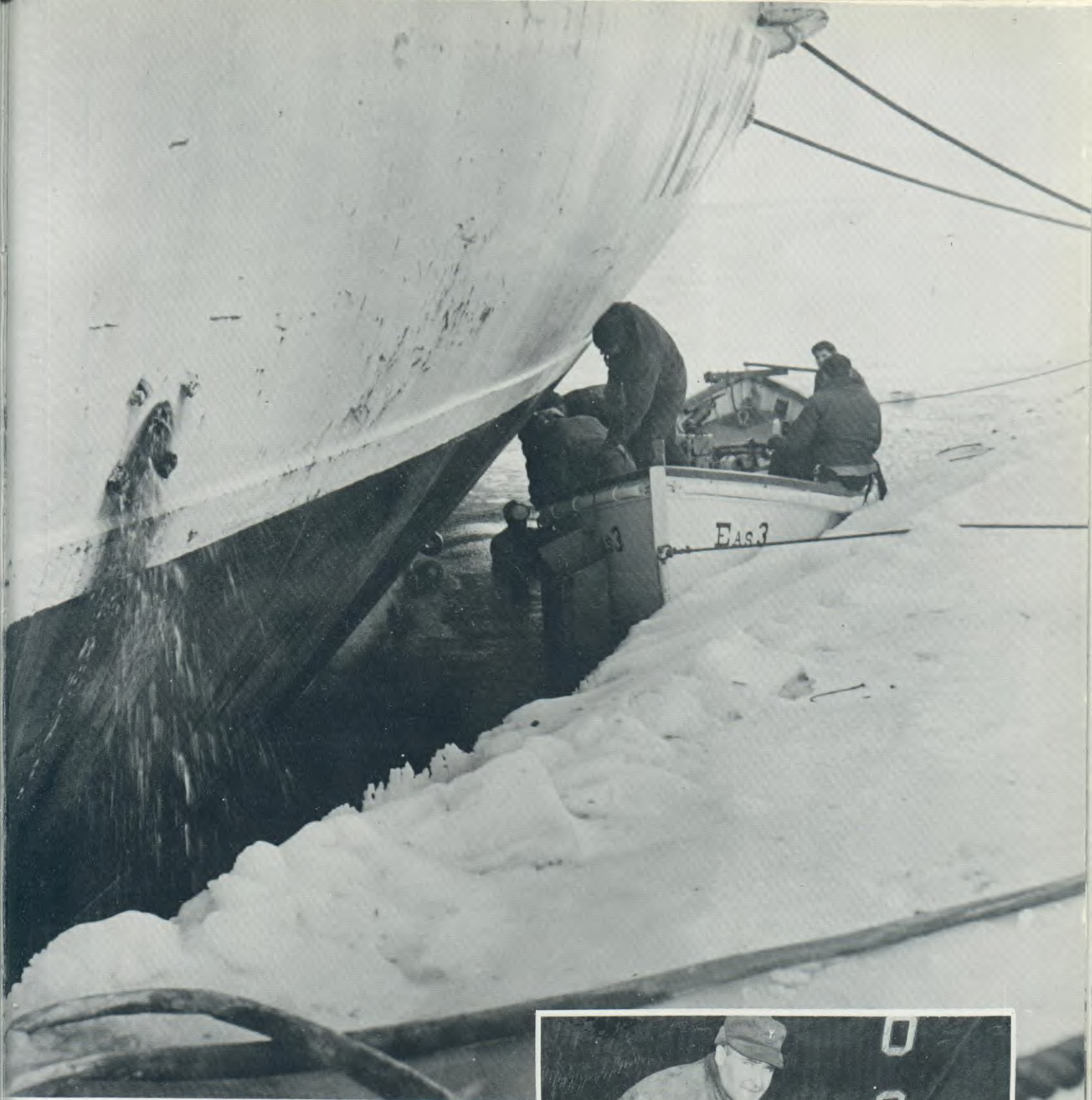
FROGMAN dives down to learn the worst. CDR Standish Backus, USN, had unenviable job of investigating damage to EASTWIND's port screw. Large photo shows general operation; insert shows CDR Backus at end of his check assisted by Robert E. Young, BM1, Coast Guardsman.
