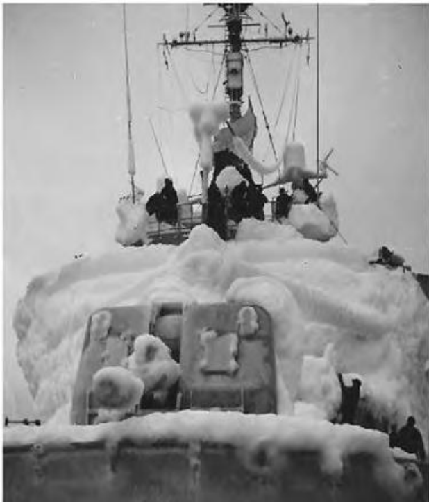
Damage to Radar and 5 Inch Gun
