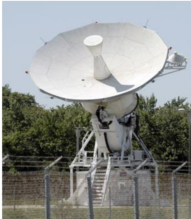
One of MILA's of two signature 30-foot steerable S-band dish antennas. Both are marked for demolition. (NASA/Kim Shiflett)
