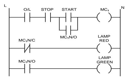
**NOTE:** It will also be accepted if both the O/L and STOP symbols are closed. NB, both O/L and STOP must be the same state.
