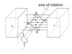
When the motor is functioning, the coil rotates in a clockwise direction as shown.
