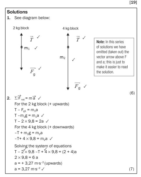
3. Option 1  $T - \left(\frac{2m_1m_2}{m_1 + m_2}\right) \times g$  $T = \left(\frac{2 \times 2 \times 4}{2 + 4}\right) \times 9,8$ T = 26.13 N Option 2  $T - F_{g1} = m_1 a$  OR  $T = m_1(a+g)$ T = 2 (3,27 + 9,8) ✓ T = 26.14 N ✓ Option 3  $-T + m_2g = m_2a$  OR  $-T = m_2a - m_2g$  OR  $T = -m_2a + m_2g$ T = 4(-3,27 + 9,8) ✓ ✓ T = 26.12 N ✓ (4)**4.** Smaller than. ✓ (1)5. Anticlockwise. ✓ (1)[19]
