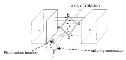
**Use Fleming's Right Hand Rule** to determine the direction of the force on the conductor –the direction in which the coil turns. Remember: the current is in the direction of the middle finger or palm, whereas the magnetic field is in the direction of the fingers (or index finger), and the thrust (motion) is in the direction of the thumb.
