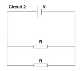
The power dissipated by each resistor in the circuit 2 is...
