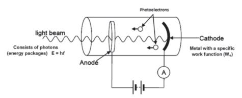
A photoelectric diode in an electric circuit
