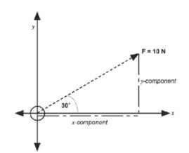
Well, the *y*-component is opposite the angle, and the hypotenuse (10 N) is known, so since sine is O/H, sin 30° × 10 N = the *y*-component: 5 N. Likewise, the *x*-component is adjacent to the angle, so since cosine is A/H, cos 30° × 10 N = 8,67 N. So your *x*-component is 8,67 N and your *y*-component is 5 N.
