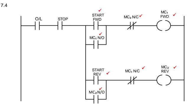
**NOTE:** - If a candidate closes the O/L or STOP inputs that were given, a mark will be deducted for each one that is closed, because the program will not operate correct according to the given diagram in the question. - If a candidate connects START REV straight to the L power rail bypassing O/L and STOP, START REV will not be awarded a mark because of the wrong connection of START REV
