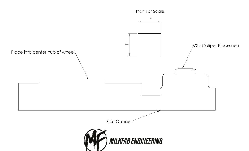
280Z Hub Z32 Caliper Front Fitment Template
