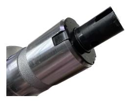
12. Install the Shaft Alignment Collar onto the end of the shaft with the side closest to the cross drilled hole towards the collar wear plate.
