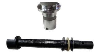
10. Insert the Milkfab shaft with the thrust assembly attached into the CSS body.
