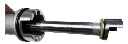
6. Remove thrust assembly and spacing washer from the Jeep Shaft/Body and place to the side (This will be reused)
