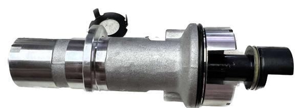
11. Place the gear/collar wear plate back onto the end of the CSS body.
