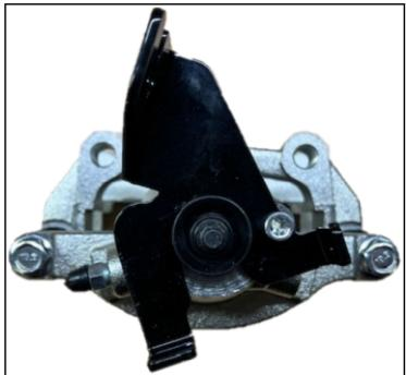
d) Swap the Ebrake actuation arm from the left side caliper to the right and vice-versa onto the center post with the "tail" of the arm resting against the stop of the Ebracket cable bracket like the original (Be sure the actuation arm is also seated in the splines on the post.) . Re-install the center nut reverse of step 10-B.
