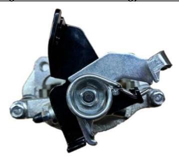
\*\*With the use of the MilkFab V2.0 Ebrake bracket the left caliper is mounted on the left side of the vehicle and the right on the right side. \*\*
