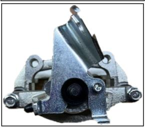
c) Remove Ebrake cable bracket mounting bolt and bracket.
