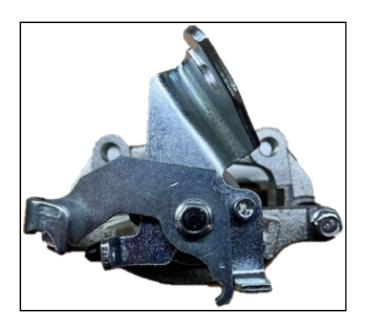
b) Remove nut from the center of the Ebrake actuation arm and remove arm. (Take note of position of the arm in relation to the Ebrake cable mounting bracket.)
