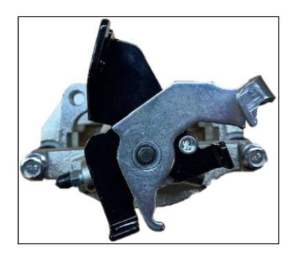
e) Re-install Ebrake return spring. The springs will also be swapped sideto-side like the actuation arm. **Be Extremely Careful Removing, Springs Contain Large Amounts of Stored Energy While Compressed.**
