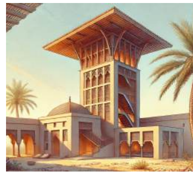
Malqaf : Towers designed to catch and direct cooler breezes into buildings while expelling hot air..
