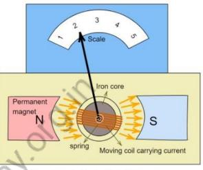
Front view of a Moving Coil Galvanometer
