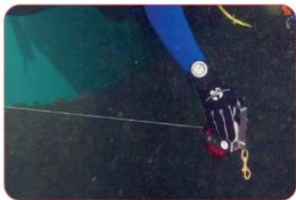
Maintain light tension on the line at all times by keeping a finger on the reel. Slack makes tangling or jamming the reel very likely.
