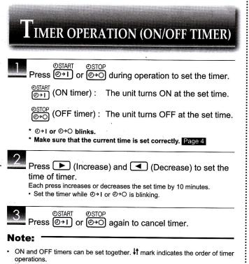
If power failure occurs while ON/OFF timer is set, see page 5 "Auto restart function".
