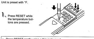
Press RESET gently using a thin instrument. To change temperature unit from °C to °F, press RESET.
