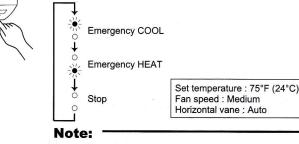
The first 30 minutes of operation is test run. Temperature control does not work, and fan speed is set to High.
