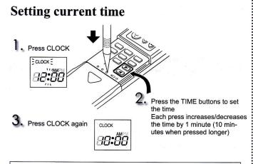
· Press CLOCK gently using a thin instrument.
