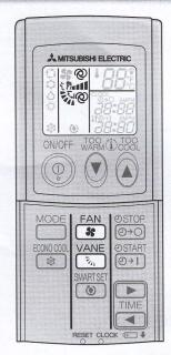
Press sto select fan speed. Each press changes fan speed in the following order:
